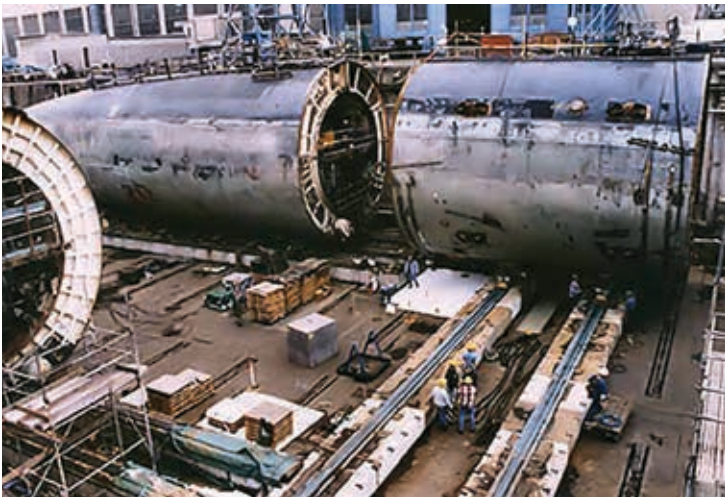
At PSNS, here we see the separation of the reactor compartment from sections fore and aft.
