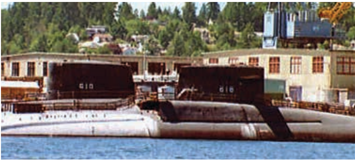
The former USS Thomas Jefferson (SSBN-618) has been reassembled following removal of the missile and reactor compartments at PSNS.
